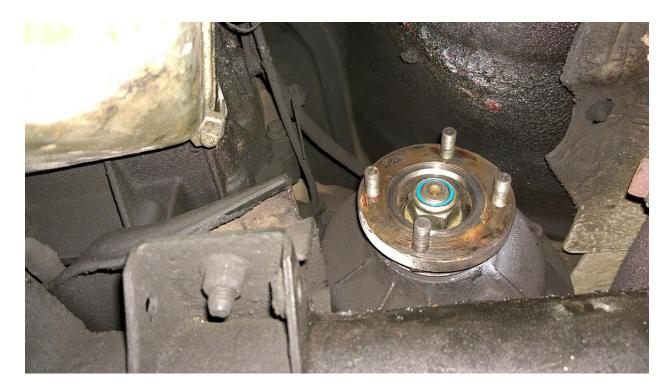
Once the shaft has been removed, you can see the flange bolt hiding above the cross member, with the viscous coupling housing behind that.
