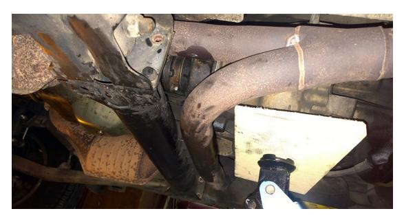
Then refit the mount bolts and nuts, torque to 33Ft Lbs (45Nm).
