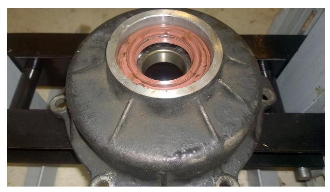
Next flip the housing over and press the new VC unit into the bearing.
