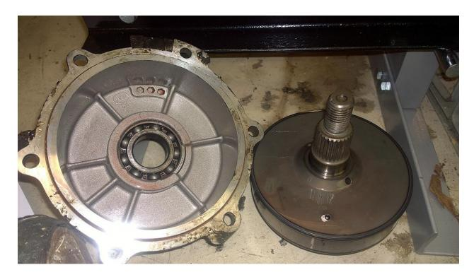
The old VC pressed out of the housing, you can see the bearing which I also replaced while I had it apart.
