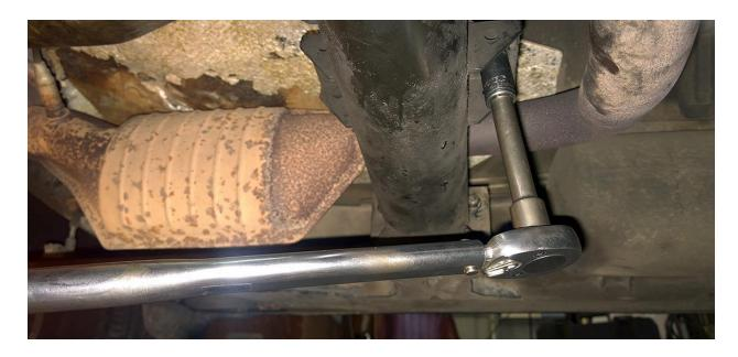
I did the snubber bar last, it goes through a hole above the center of the cross member, the 2 bolts thread into each end of it.
