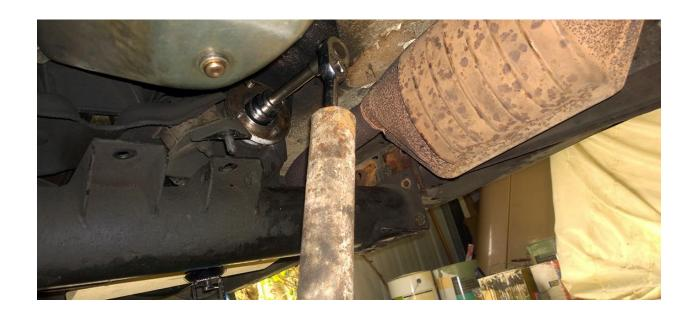
Next step is a 75mm gear puller to remove the flange. Mine came off pretty easily.
