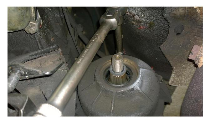
Next remove the 6 bolts around the vc housing. 15mm socket required and maybe an open end spanner for the left most bolt which is in a tough spot.
