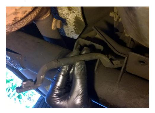
Next remove the jack that was supporting the transmission, then attach and tighten the drive shaft flange bolts at front and rear. You will be getting tired at this stage, be patient, you are nearly there! Again I ended up rolling the vehicle forward to access each nut in turn.
