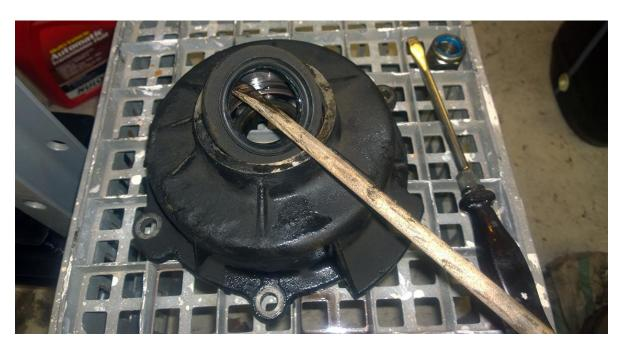
I replaced my output bearing as well while it was apart. The bearing had some movement, so it was a good opportunity. Some circlip pliers are needed to remove the large circlip that holds the bearing in place.
