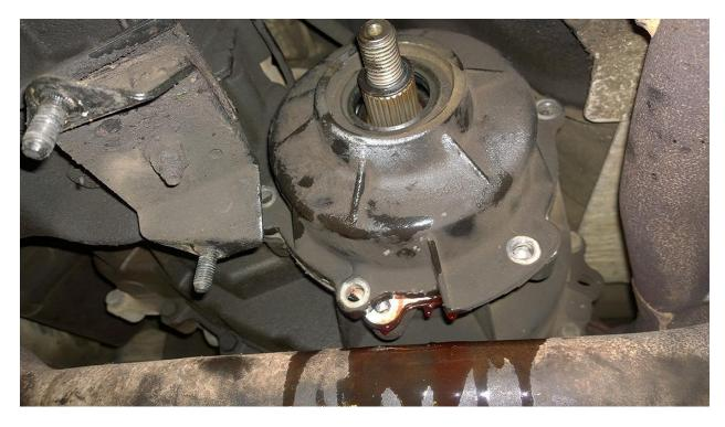
I had to give the VC shaft a few taps on the sides, top and bottom with a hammer to get it to release from the shaft. Once released it comes off easily.
