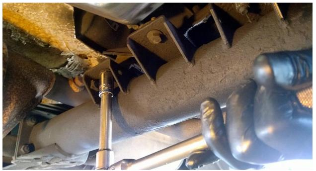
15mm socket with an extension needed here. The 2 middle bolts are attached to a small 'snubber' bar, which fits over the top. It comes out easily once undone.
