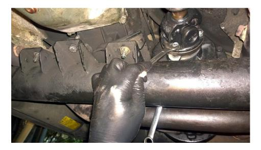
Last but not least, refill the transfer case with correct ATF and refit the plug.
