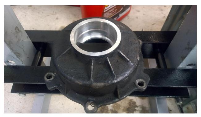
Next press in the new bearing on the outer race only, you can damage the bearing if you press the center part.
