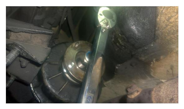
Next I located the drive shaft onto the flanges, loosely doing up a couple of bolts on each end so it didn't fall off. I figured it was easier to do that before the cross member went back on.
