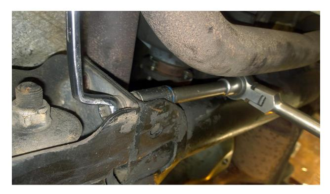
13mm ring spanner on the bolt end here, 15mm socket on the nut. Once everything is undone, it will require some gentle persuasion with a heavy hammer to get it moving. It will move fairly easily, just ease it out as straight as you can at both ends. It's not very heavy to handle once it's off.
